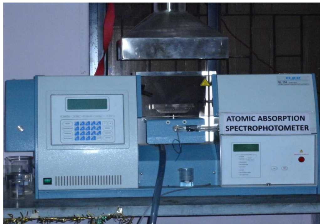
Atomic Absorption Spectrophotometer machine to test micro nutrients level in soil samples
